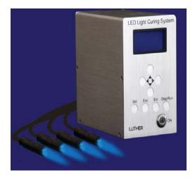
One of the biggest benefits of using the LED technology is that the light source life is much longer than lamps used in lamp type UV systems. The life of the lamp type is approx. 3,000hours, but the LED has approx. 20,000 hours. Further more, unlike the lamp type, which needs to be kept turned on through out the operation, the LED can turn on instantly only when it is needed.
