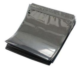
Surface Resistance:  $10^{-10^{10}}$ Metal layer resistance:  $<100 \Omega$ Metal layer optical transmission:  $40^{-70}$ Seal: Heat Seal Hot sealing temperature: 250-375FColor: Silver Grey Thickness: 2-4 mil Tear Resistance: 20 lbs Puncture Resistance: 30 lbs Static Shielding: 20 volts Static Decay: <0.03 seconds Certificate: Rohs Size: Customized
